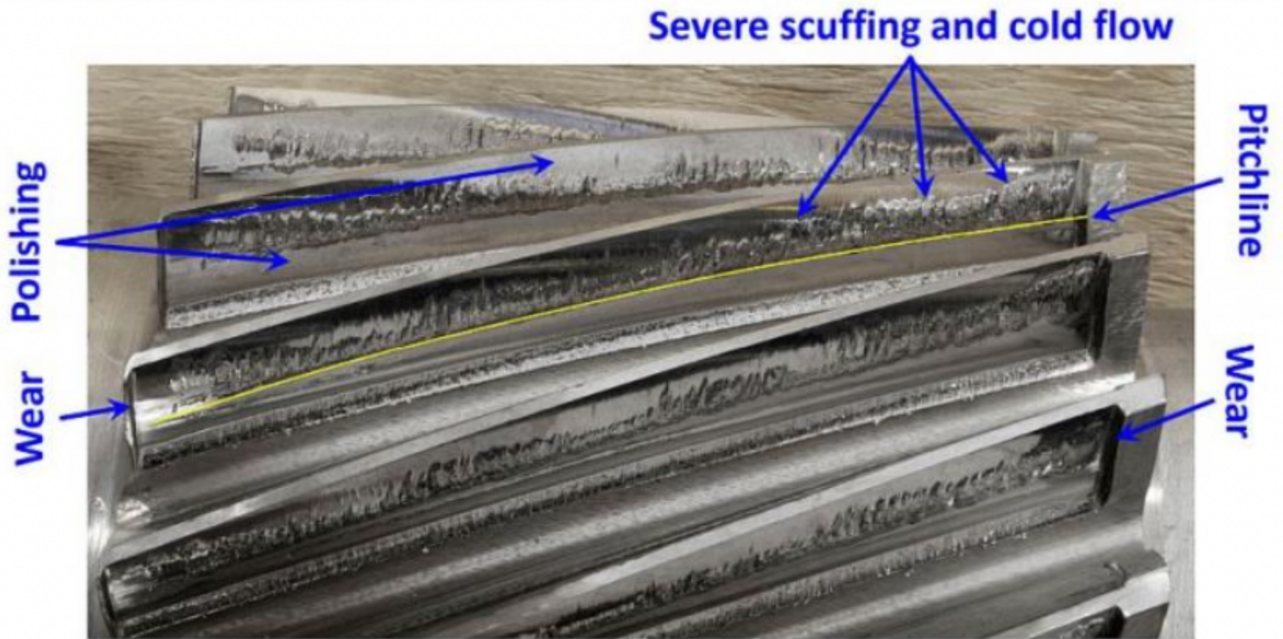
Figure 6: Adhesion between gear teeth resulting in scuffing.
