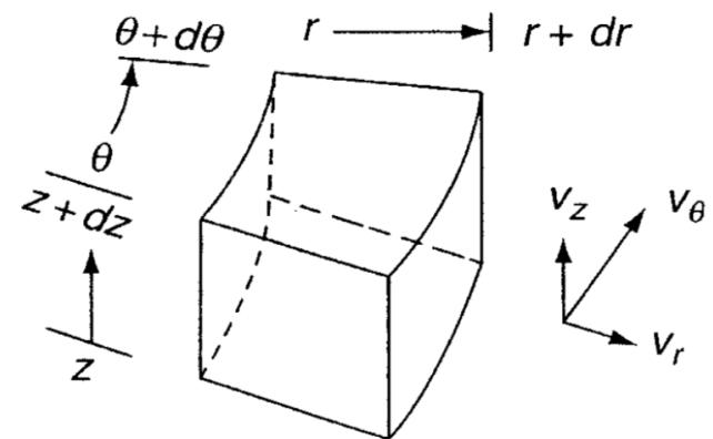
$$\dot{m}_{in} - \dot{m}_{out} = \frac{\partial}{\partial t} m_{element}$$
