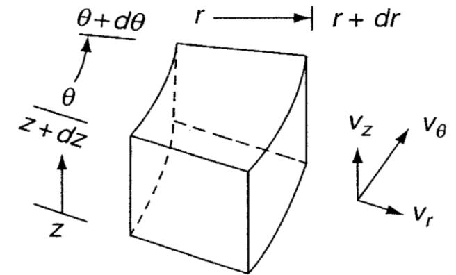
For 2-D incompressible fluid, there is no changes in density and velocity for z-direction is zero.
