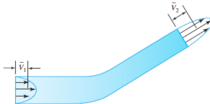
Figure 4.7 Nonuniform velocity profiles.
