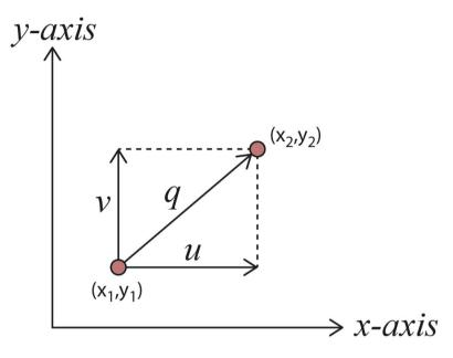
u = Velocity on x direction v = Velocity on y direction q = Resultant velocity
