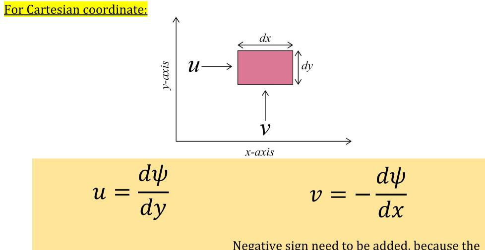
Negative sign need to be added, because the rotation direction is counter-clockwise.
