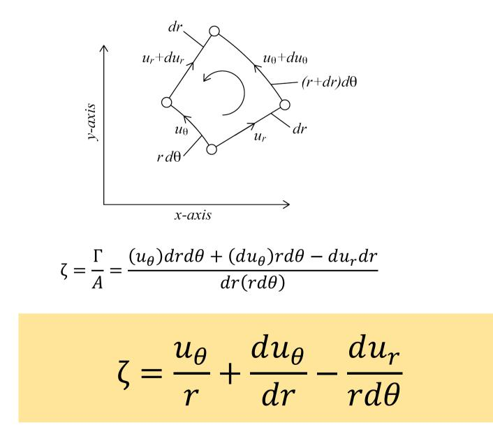
Not like continuity equation, vorticity is not always equal to zero.  $\frac{du}{dx} + \frac{dv}{dy} = 0$
