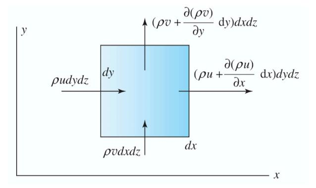
The net flux of mass entering the element equal to the rate of change of the mass of the element.
