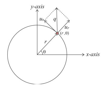
$u_r$  = Velocity on radial direction  $u_{ heta}$  = Velocity on angular direction q = Resultant velocity
