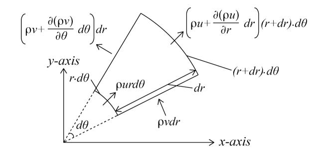
The net flux of mass entering the element equal to the rate of change of the mass of the element. Assume that z-direction is equal to 1 unit.
