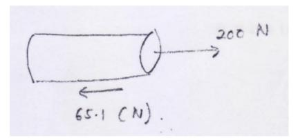
Total pulling force = Drag force at side + Drag force at front surface
