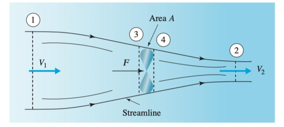
This control volume is not sufficient, however, since the areas  $A_1$  and  $A_2$  are unknown. We know the flow area A of the propeller.
