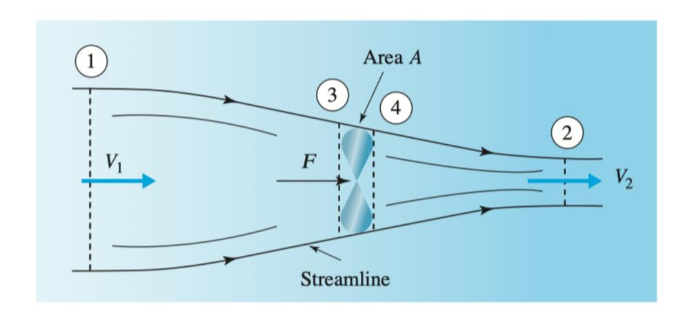
This control volume is not sufficient, however, since the areas  $A_1$  and  $A_2$  are unknown. We know the flow area A of the propeller.
