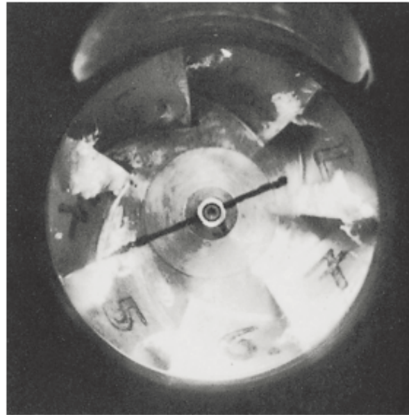
Figure 12.10 Cavitation bubble distribution in an impeller region. (Courtesy of Sulzer Pumps Ltd.)
