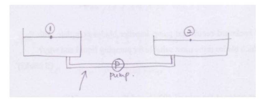
f = 0.05 l = 1km D = 0.15m pump power = 80kW
